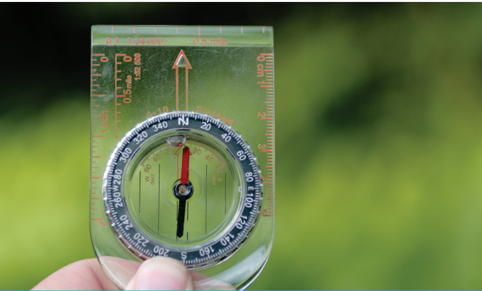
When bearings are expressed in degrees, north is defined as 0 degrees, and the number of degrees begins rising with bearings that lie to the west of north, moving 360 degrees through east, south, west and back to north at 0 degrees.
